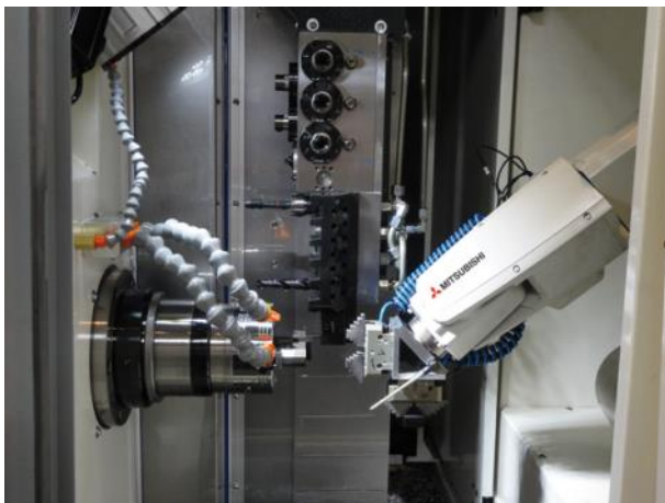
Picture 3: The RV-6SD 6-axis robot from Mitsubishi Electric is also completely integrated in the iRobo from müga which enables considerable savings on space to be made. The machine has turning, milling and drilling functions so that it satisfies the customer's requirements for complete machining.
