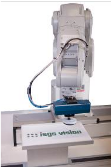
Picture 2: RoboView 3D from isys vision allows Mitsubishi Electric robots to alter their predefined paths to see the room and act adaptively.
