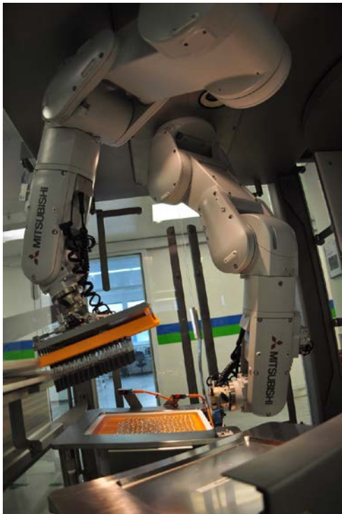
Picture 3: The special feature of the syringe handling solution is not only having the MELFA robots suspended overhead but also having two working together in the minimum of space.
