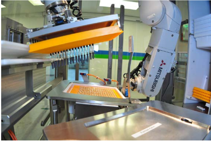
Picture 2: The syringe handling solution can index 400 syringes per minute in the emptying rail. An additional axis enables the solution to handle up to 600 syringes per minute.
