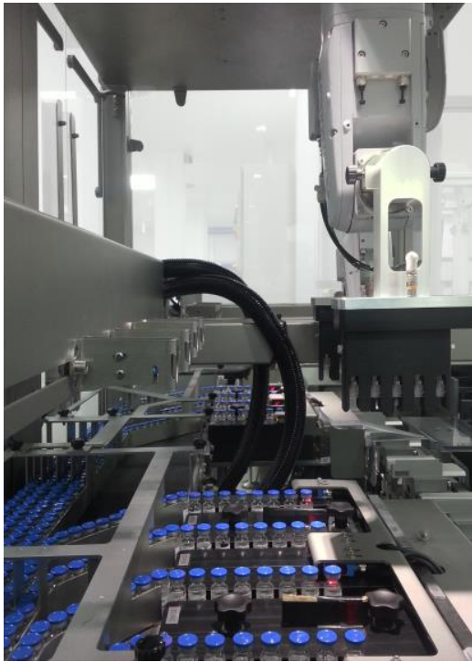
Picture 4: The MELFA RV-4FL robot uses vacuum grippers to lift two rows of five vials each from the positioning screws and put them into the waiting packing units.
