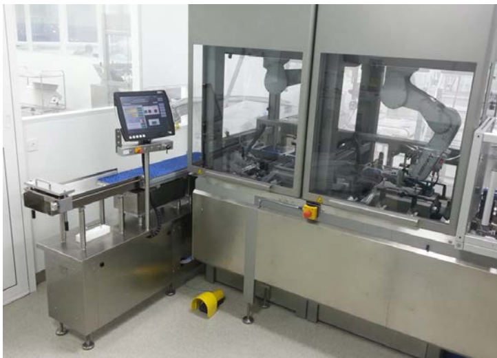
Picture 5: The vials handling solution essentially consists of two MRT cells each with an overhead articulated-arm robot from Mitsubishi Electric and a conveyor system equipped with Mitsubishi Electric servomotors.
