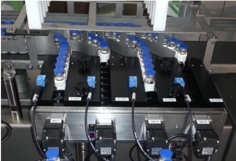
Picture 2: The dynamics of the Mitsubishi Electric servos come into their own especially in the conveyor system, due to fast acceleration and high braking torques combined with a very gentle start-up and deceleration.
