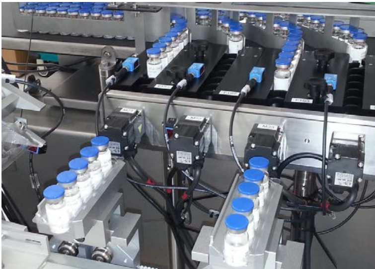
Picture 3: One MELSERVO MR-J4 servo motor drives a positioning screw in each case, indexing the small bottles into the lanes and readying them in groups of five.
