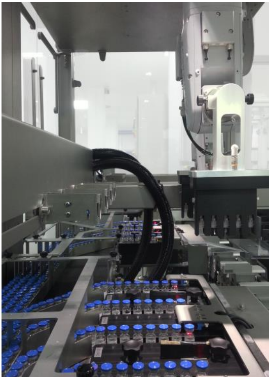
Picture 5: The MELFA RV-4FL robot uses vacuum grippers to lift two rows of five vials in each case from the positioning screws and place them in the waiting
