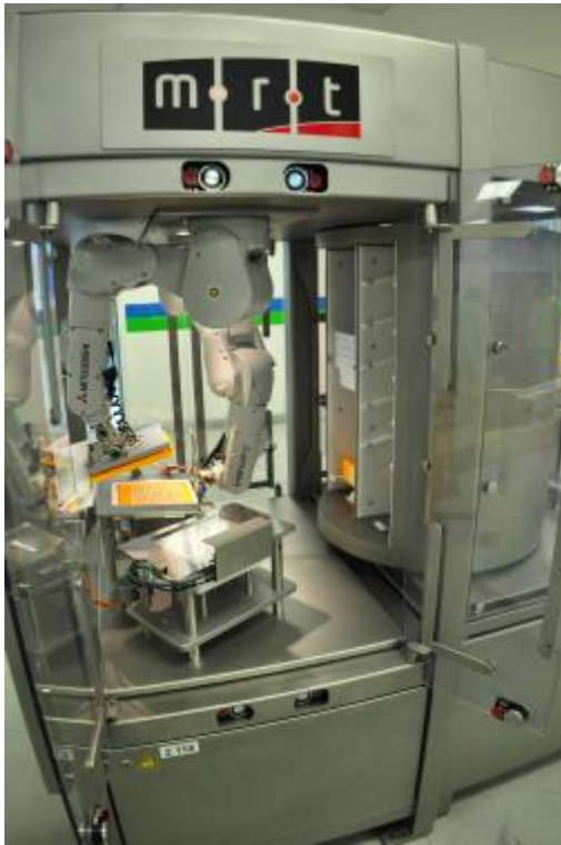
Picture 6: Two Mitsubishi Electric robots type MELFA RV-4FL are used in the handling solution, working together in the limited space. The rotary turret (right) conveys the tubs loaded with the syringe carriers to the MRT.
