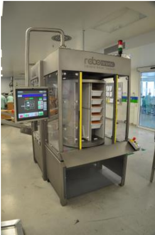
Picture 4: The turret in the application holds ten tubs in all and has to be reloaded every four minutes. To achieve the same autonomy with a conveyor belt, the belt would have to be four metres long.
