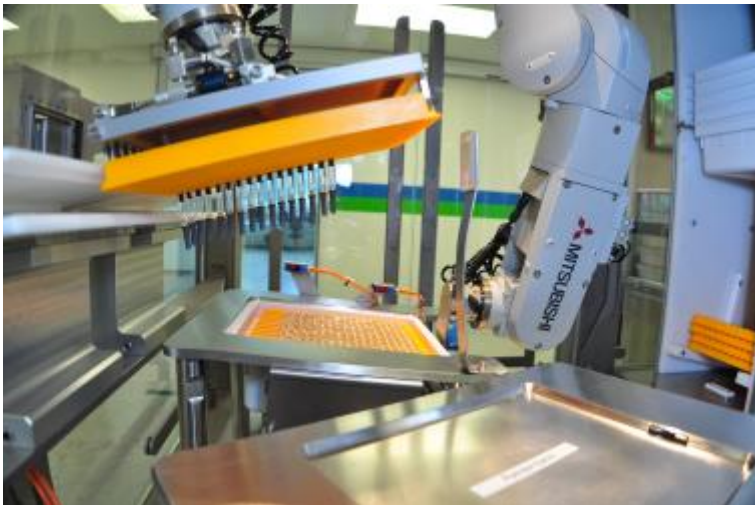
Picture 10: The syringe handling solution can index 400 syringes per minute into the emptying rail. Adding another axis means that this solution can process up to 600 units per minute.
