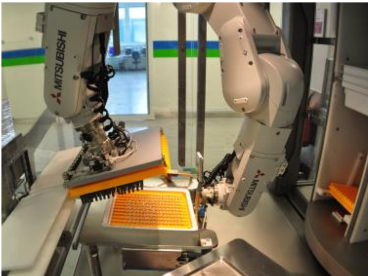
Picture 8: A switching option facilitates a rapid change between the two carrier formats and between different syringe formats ranging from 0.5 to 10 millilitres.
