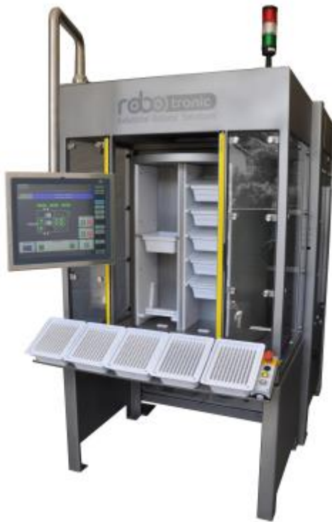
Picture 3: Instead of a conveyor belt extending over several metres for supplying the tubs, Robotronik has developed a rotary turret, which is based like the robot cell on a space-saving MRT module.
