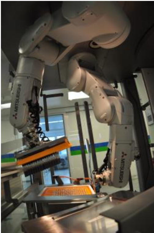
Picture 7: The special feature of the solution is that the robots are not only suspended overhead, but work in pairs in the minimum of space.
