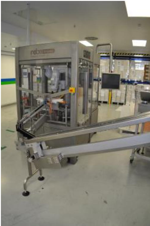
Picture 5: From the emptying rail the syringes move to the final packaging system.
