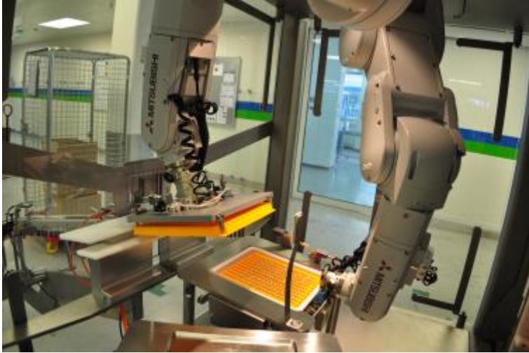
Picture 9: The two MELFA robots assume responsibility for the overall handling of tubs, carriers and different syringe formats.
