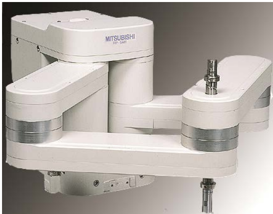
Figure 2: The Mitsubishi Electric dual-arm SCARA robots from the RP series are compact high-performance systems specially designed for micro-handling.
