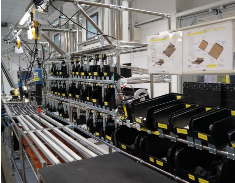
Picture 3: HMIs replace static assembly instructions with dynamic screen information that can provide live assembly instructions and performance data.
