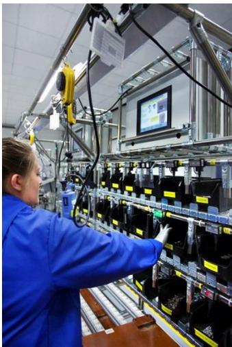
**Picture 2:** The variety of operator guidance devices ensured that a wide range of picking scenarios could be accommodated and tested.
