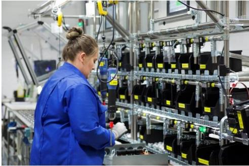
**Picture 1:** The simple but effective Guided Operator Solutions from Mitsubishi Electric, Factory Automation ensures the correct part is selected.
